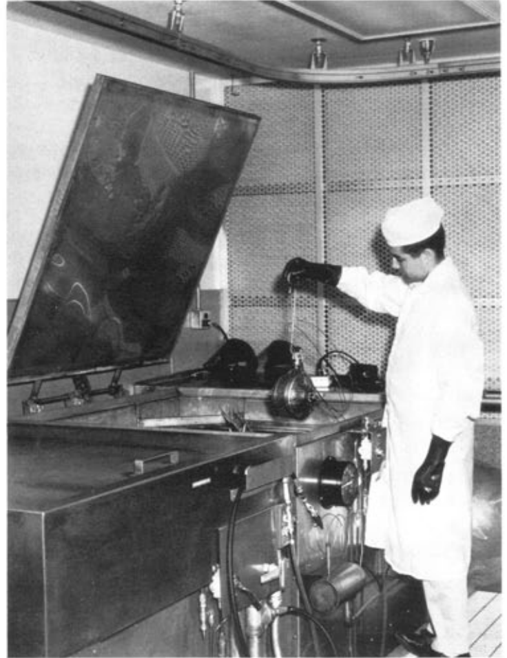
ALL MATERIALS THAT ENTER THE CLEAN ROOM FOR ASSEMBLY ARE FIRST CLEANED IN THIS PRE-CLEAN AREA. A WORKER IS SHOWN ABOVE REMOVING A PART FROM ONE OF A SERIES OF SIX FIVE-FOOT DEPTH TANKS WHERE PARTS ARE DEGREASED AND CLEANED. AN OVERHEAD MONORAIL ALLOWS INTRODUCTION OF VERY LARGE OBJECTS INTO THE CLEANING TANKS.
